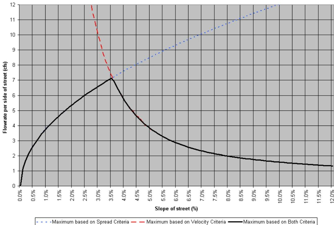
Note: The spread of water in the street is calculated using the Manning equation in the form developed by Izzard, with a roughness coefficient of 0.013 and the standard street cross section. The velocity criteria is based on the velocity at the deepest part of the gutter with the Manning Equation, with a roughness coefficient of 0.013, and using a depth at a point six inches from the face of the curb as the hydraulic radius.
